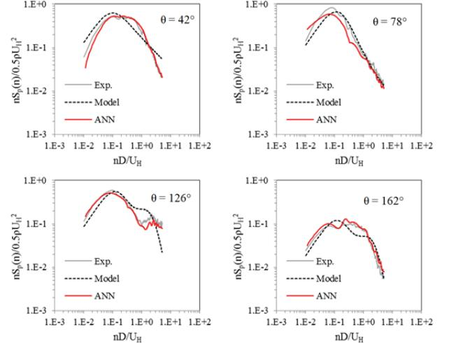
Figure 4. ANN prediction, approximation formula and experiential spectra of the F4 validation case at 4 different tap locations
