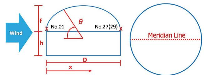
Figure 1. Geometric nomenclature and coordinate system
