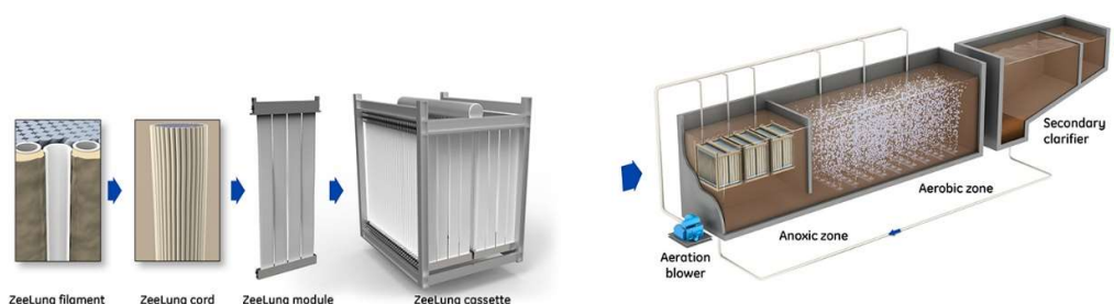
Figure 1 a) MABR system and b) MABR cassettes submerged into anoxic tanks obtained from SUEZ Zeelung website ("Zeelung Membrane Aerated Bioreactor for Wastewater | SUEZ," 2021)
