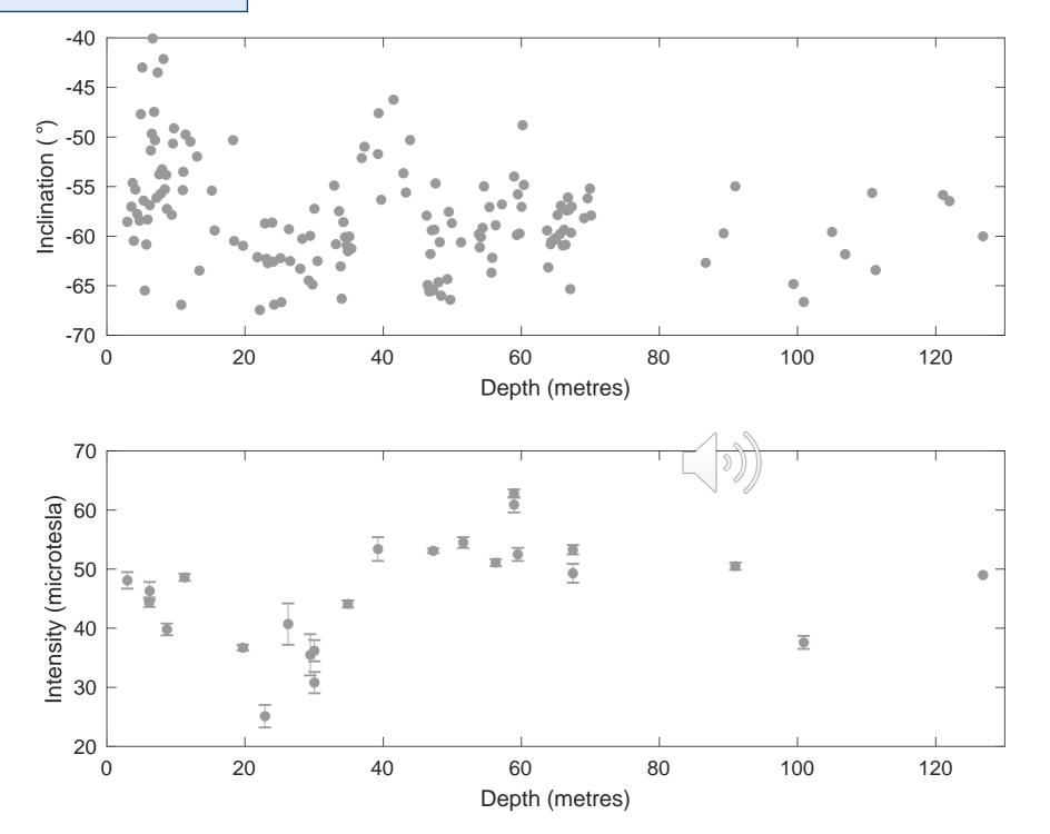
High inclination and high intensity values are observed at around 40 metres and 60 metres depth.
