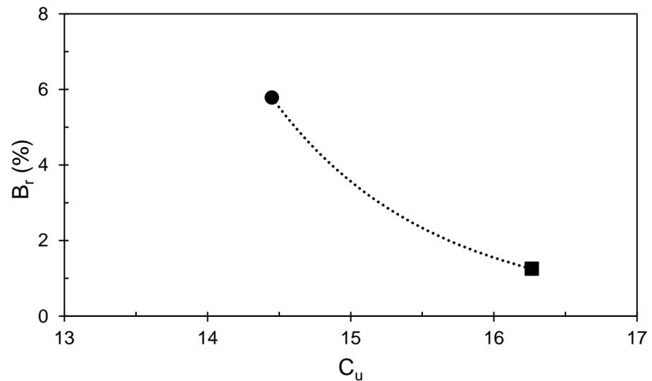
**Kaharoa less weathered** and relatively **coarser** than **Maungataketake**, shows **lesser breakage** upon compaction
