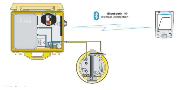
Figure 2. The portable soil gas equipment set up. The orange box is mounted on a backpack frame and contains the LICOR 820 sensor, battery, wireless transmitter and pump. This set up may be used with a soil gas  $CO_2$  probe for  $CO_2$  concentrations as well as the accumulation chamber for  $CO_2$  flux.
