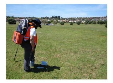
Figure 7. Measuring soil gas  $CO_2$  fluxes in Lloyd Elsmore Park, Auckland, an urban area overlying a suspected fault, a possible fracture connecting warm water to the surface, and a potential volcanic lineament. Soil gas concentrations were not measured at this site.
