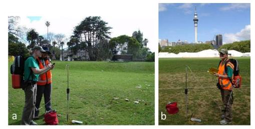
Figure 5. Measuring soil gas CO<sub>2</sub> concentrations and fluxes in a) Albert Park and b) Victoria Park, two urban, no fault settings in Auckland. Soil gas fluxes were also taken at these locations.
