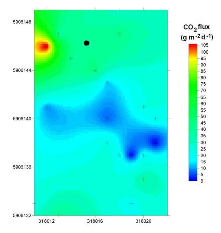
Figure 17.  $CO_2$  flux map around the Whitford well at Site 6. The black point is the site of the well. The measurement locations are represented by crosses.
