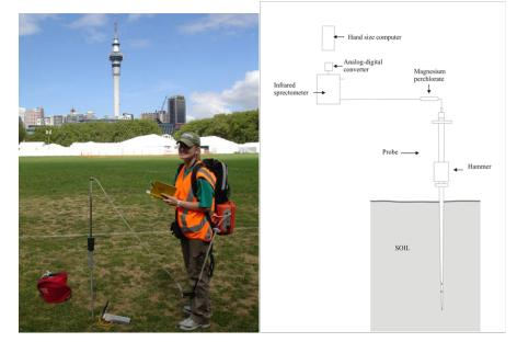
Figure 3. Measurement of soil gas  $CO_2$  concentrations in Victoria Park, Auckland. The perforated probe is inserted into the ground and tubing attached to a Mg(CIO<sub>4</sub>)<sub>2</sub> water scrubber, then connected to the LICOR sensor, pump, and battery setup in the backpack. The LICOR system was controlled wirelessly using a handheld computer. Soil temperatures were taken at each site (instrument near soil gas probe).
