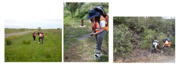
Figure 8. Measuring soil gas  $CO_2$  flux measurements in a) Puhunui Reserve (5), b) next to a warm water well in Whitford (6), and c) on Rangitoto Volcano (7). These sites represented rural, fault areas in the study. Soil gas concentrations were not measured at these sites due to time and pedology constraints.
