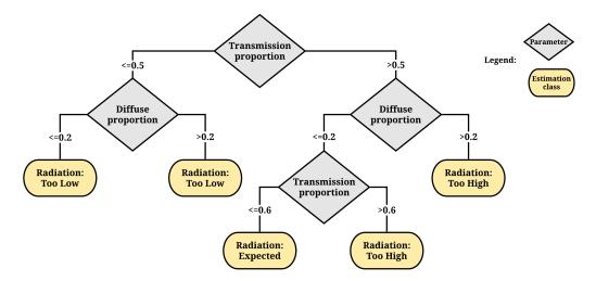
Figure 5: Decision tree diagram for parameter-setting support
